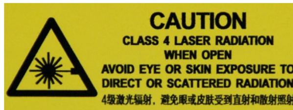
This symbol indicates laser radiation. We place this symbol on products which have a laser output.
